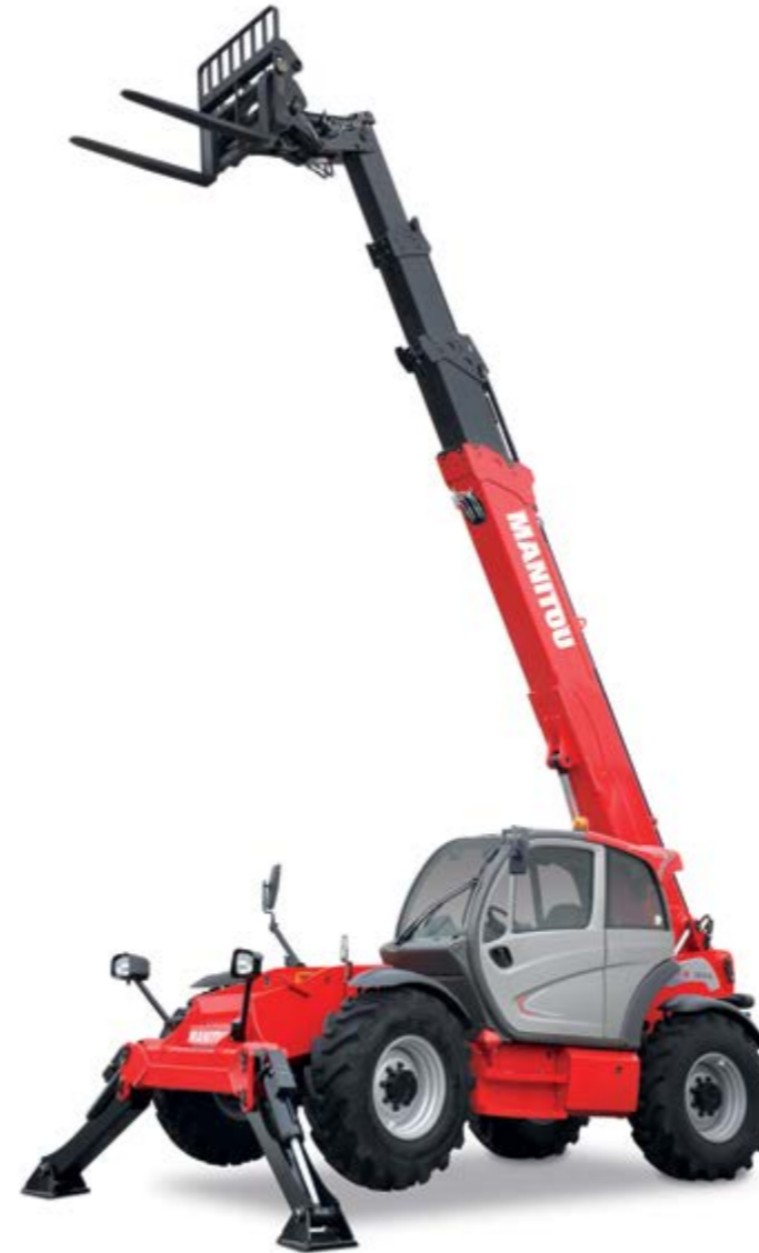
Machine on stabilizers with forks Stability norm ISO 22915-14
