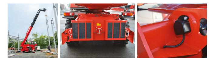
MRT-X 2470 and 3050 models sit on stabilisers equipped with strain gauges for greater precision in all surfaces.
